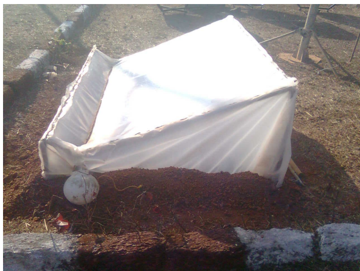
Plate: 6. Single sides (L shape) solar still.
