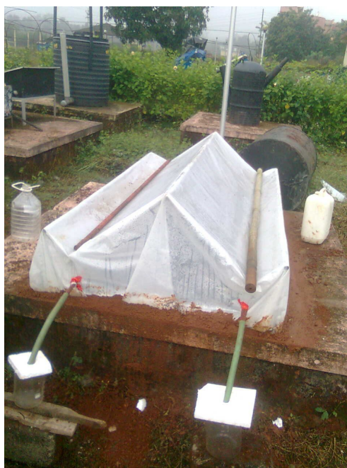
Plate: 5. W-shape solar still on concrete with two channel
